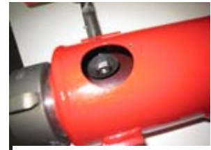
Splash guard aligned using pitot shaft.
